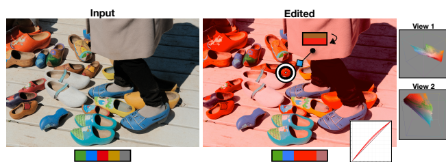
Fig. 7. ColorfulCurves operates in Lab-space, whose gamut is larger than RGB. In this example, a single image-space constraint is placed changing the brown shoe to an extreme red. ColorfulCurves clips the resulting pixel colors lying outside the RGB gamut. Right: Two views of the clipped colors in RGB space.
